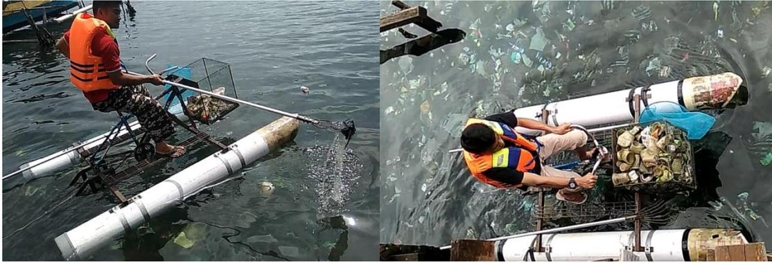
Figure 5. Bike movement and garbage transport testing
